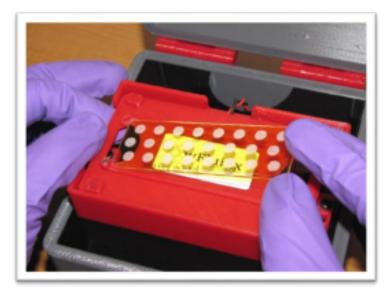
4. Ensure that the chip is securely held flat by the platform; within the ridges.
