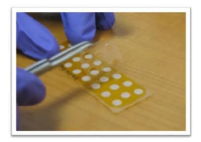
3. Load the chip into the chip holding platform with the roughened chamber circles facing upward. When loading the chip, place the chip in with one side in first, followed by rest of the chip as shown in figure on the right. Be careful not to overstress the springs suspending the platform through excessive compression or stretching (the protective red guard will inhibit some of these stresses). Holding the platform steady with your other hand could be useful in this case.
