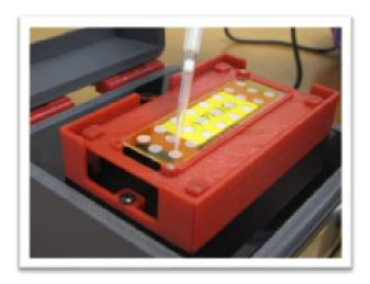
11. Remove the chip from the platform by pressing up on the bottom surface of the chip through the holes in platform. The base unit can now be powered off and the base unit lid can be closed to protect the platform if no further embryos need to genotyped.
