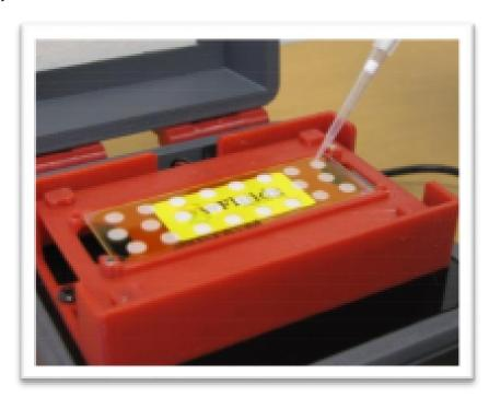
6. Place the platform lid on the platform. The lid will temporarily affix itself to the platform by magnetic forces and also firmly hold the chip on the platform. In addition, the lid would inhibit loss of media (due to evaporation) from the loaded chambers during DNA extraction.
